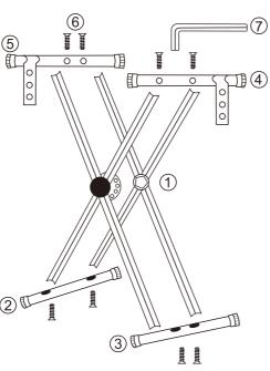
1.respectively.put the bracket foot ② and ③ in the position of the direction shown in the figure . using the tool ⑦ tighten the screws ⑥ on the X bracket ① 2.respectively.put piano upper rack beam ④ and ⑤ in the direction shown by picture . withttools ⑦ . fastening screws ⑥ X Bracker ④ on.
