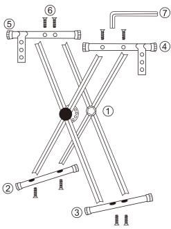
1.respectively.put the bracket foot ② and ③ in the position of the direction shown in the figure . using the tool ⑦ tighten the screws ⑥ on the X bracket ① 2.respectively.put piano upper rack beam ④ and ⑤ in the direction shown by picture . withttools ⑦ . fastening screws ⑥ X Bracker ① on.
